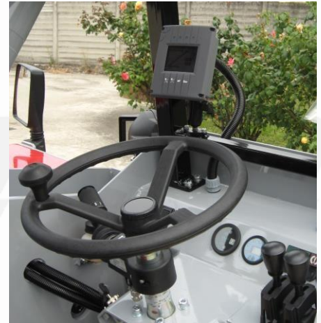
Operator's cabin with ergonomic controls and digital display for the electronic load moment indicator
