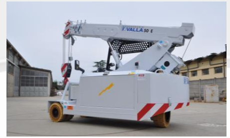
Rear steering with 180° rotation for maximum manoeuvrability
